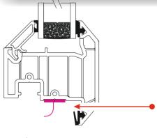
Fit a Sash Spring to the sash on the center line of the stay fixing area
