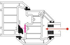
It may be necessary to pack the sash/glass at this point as shown
